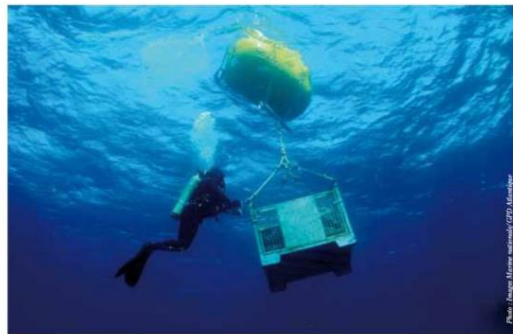
Securing and raising the container to the surface 固定及拉升貨櫃至水面
